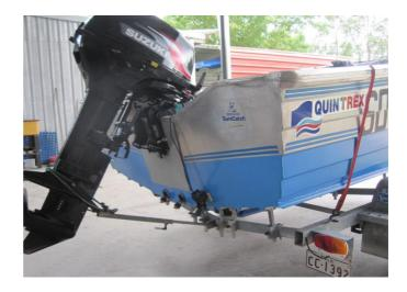
Start by removing the engine from the transom, in this case a 1 inch block was spacing the outboard up, remove this at the same time.
