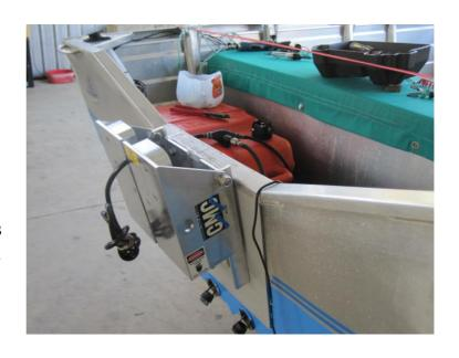
At this stage I like to drill a 3-4 mm hole in the plate so that a zip tie can be used to hold the electrical lead in position.
