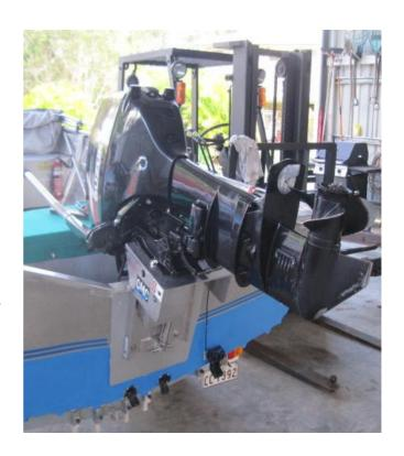
Now tilt the outboard back down again so that you can easily drill through the trim and tilt plate, using the outboard as a template.
