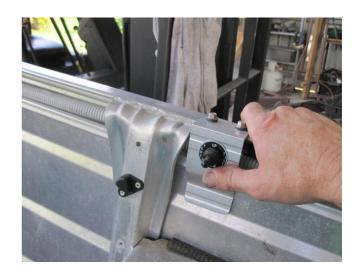
Now your PT-35 is all mounted up and ready to have the outboard fitted. At this stage you would have finished mounting the switch, positioned the relays and extra wiring in the battery box, or where-ever you decide to place it.
