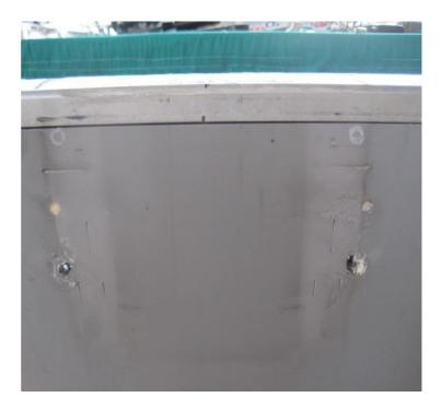
Once you have your bolt holes drilled, fit the bolts, place the unit into its correct position, tighten the bolts using nylocks or stainless spring washers. I used a strap washer with nylocks for the top fasteners in this case, it lends support and makes a neat job.
